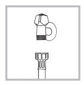
1. Connect the supply pipe by screwing it to a cold water tab using a ¾ gas threaded connection (see figure).
